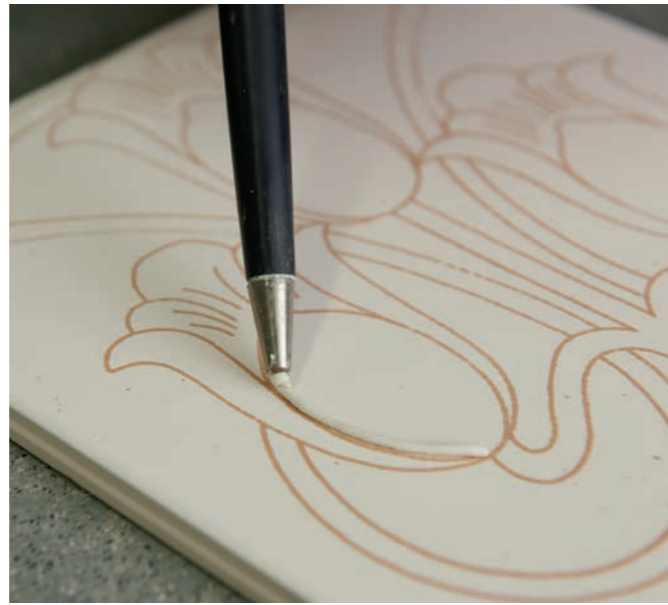
2. The pattern is stencilled onto the blank tile biscuit (this one is Liberty). A thin line of slip is carefully piped following the stencil lines – just like icing a cake
