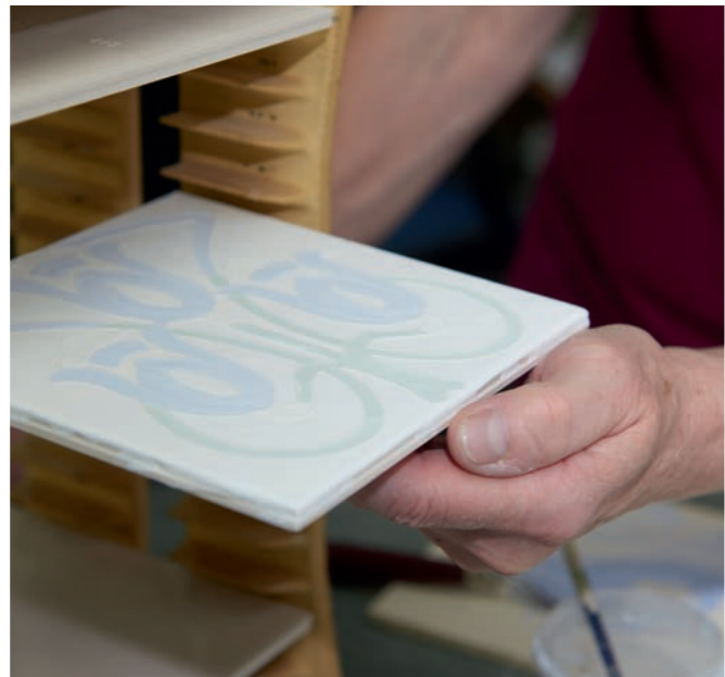
4. When all the colours have been applied, the tile is inspected, loaded into a crank and then left to dry, before being fired in the kiln
