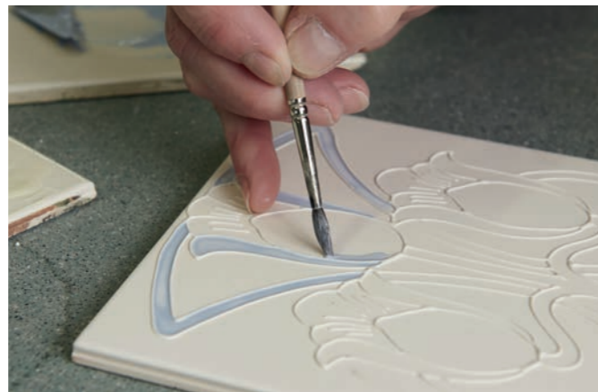
3. When the piped outline has dried, coloured glazes are hand painted in separate areas within the lines. As you can see, the glaze colour does not resemble the finished tile
